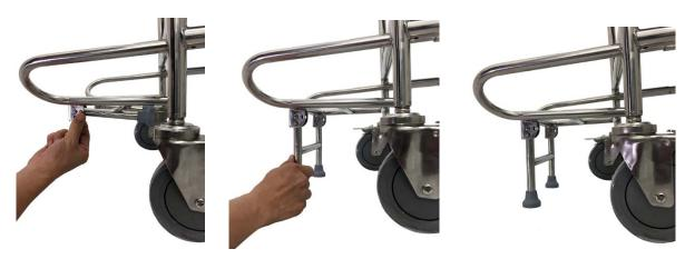
Press the side button to release the lock. Pull the front anti tipper downwards and lock into vertical position for use.
