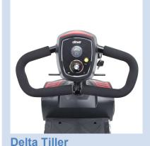
Wrap-around delta tiller allows driving by one hand
