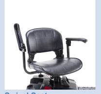
Swivel Seat 360° swivel seat with flip-up armrest makes it easier to get on or off the scooter
