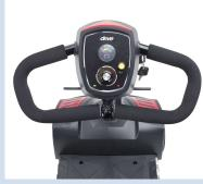
Delta Tiller Wrap-around delta tiller allows driving by one hand
